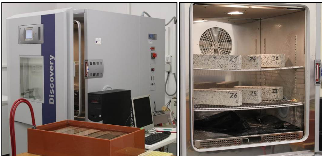
Figure 2.: Apparatus for cyclic freezing and thawing of specimens.
